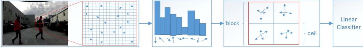
Fig. 3. The pedestrian detection process of a monocular camera. Step 1: calculate pixel gradients, i.e., magnitude and direction in 8x8 cells. Step 2: each pixel votes for its cell gradient orientation depending on its gradient magnitude. Step 3: concatenate cell histograms into blocks of 2x2 that describe the final HOG feature vector of the whole image. Step 4: classify resulting HOG feature vector into pedestrians and other.
