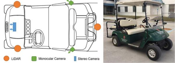
Fig. 2. Experimental vehicle (right) and the configuration of on-vehicle sensors (left).
