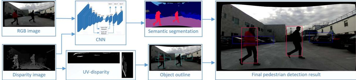
Fig. 4. Stereo vision based pedestrian detection. The top row shows the process of semantic segmentation while the bottom row shows the process of UV-disparity map based object detection.
