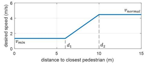
Fig. 12. The action strategy of the autonomous vehicle for the time-to-pass case. In our simulation,  $d_1 = 6$ ,  $d_2 = 10$ ,  $v_{normal} = 10\text{mph}$ , and  $v_{min} = 3\text{mph}$ .
