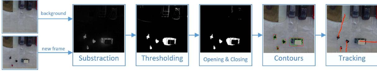
Fig. 7. Pedestrian detection of UAV-based infrastructure camera. In the scenario, 3 pedestrians are walking in shared space while the vehicle tries to traverse.
