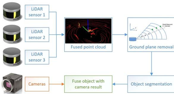
Fig. 5. The flowchart of LiDAR based pedestrian detection.
