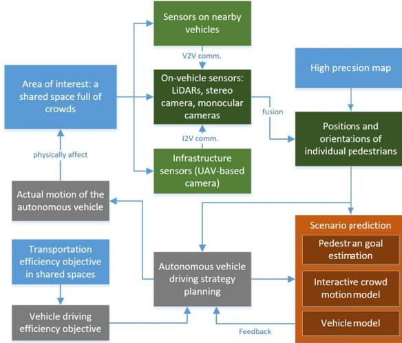
Fig. 1. The proposed framework to improve transportation efficiency.
