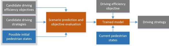
Fig. 10. Offline driving strategy determination process.
